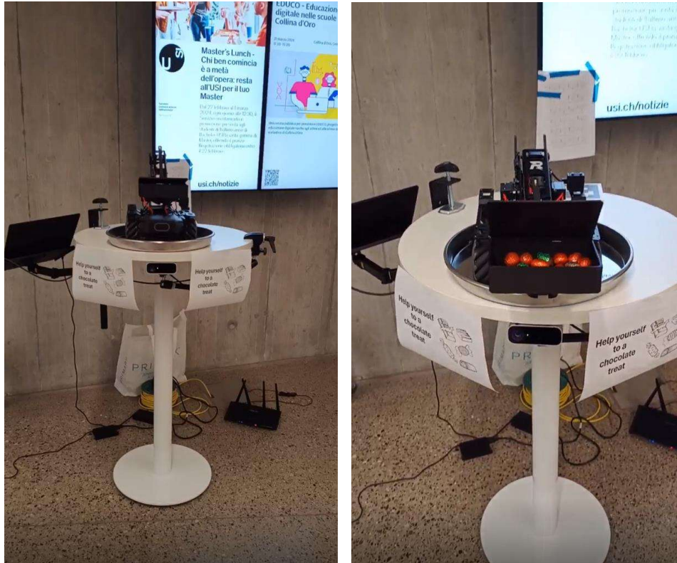
Fig. 9. Updated version of the waiter robot. On the left the rest position, on the right the offering position with the tray open and chocolate treats visible.
